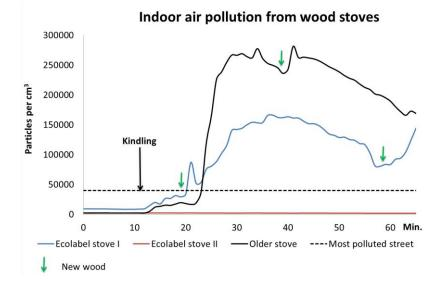
Figure 3: Indoor air pollution from different wood stoves (particles per cm<sup>3)</sup>
